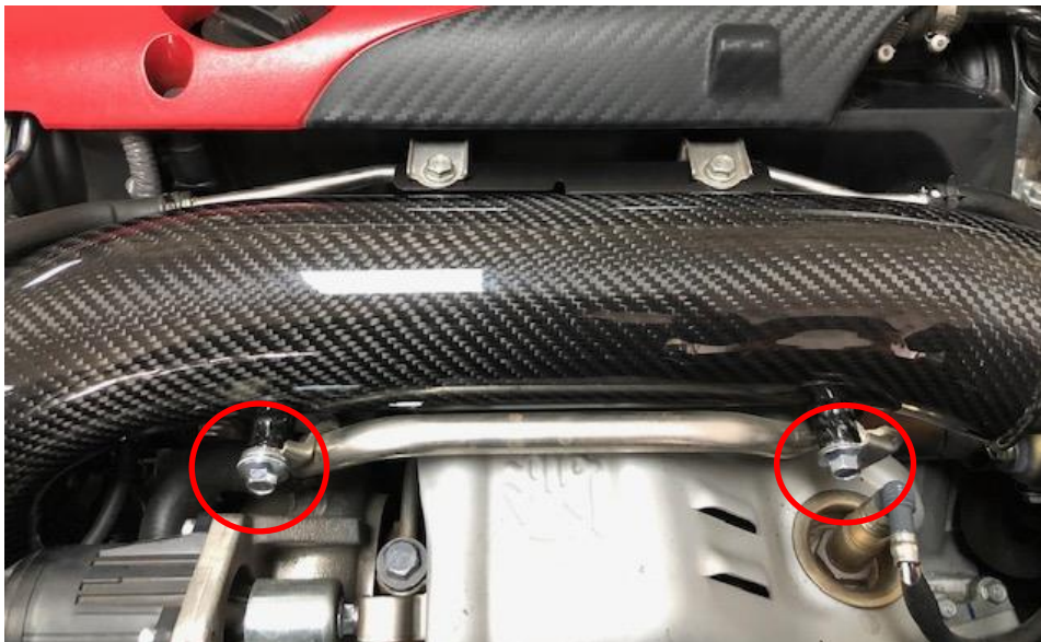
31. Secure the front metal line to the front of the tube with the supplied M6 x 10mm bolts.
