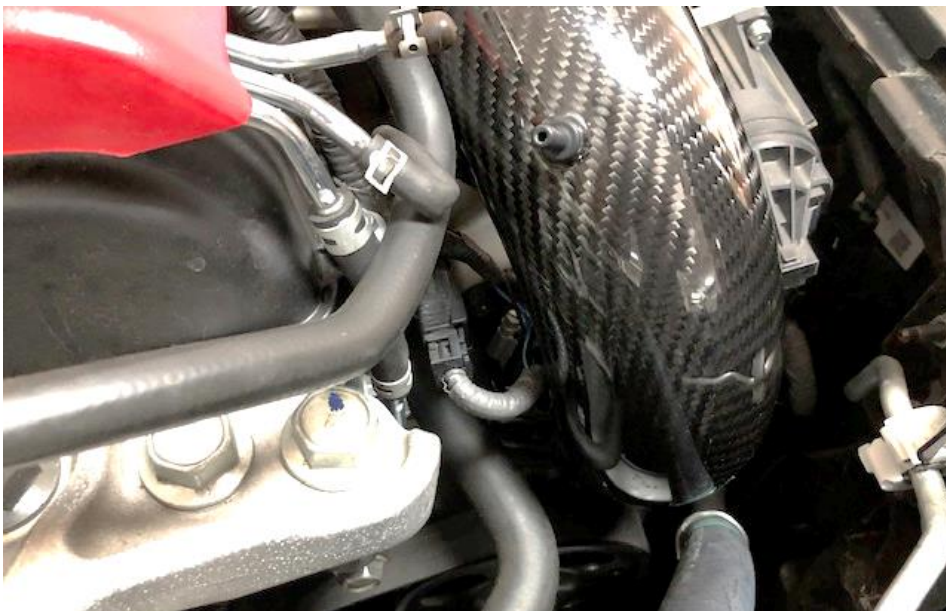
27. The wiring loom and vacuum hose should be routed to the inside of the tube. Push the tube into the silicon coupler at the turbo side. Make sure it is fully in place inside the coupler.
