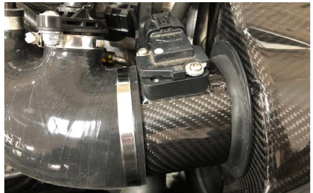
36. Ensure the carbon MAF tube is pushed into the silicon as far as possible. Secure all hose clamps.
