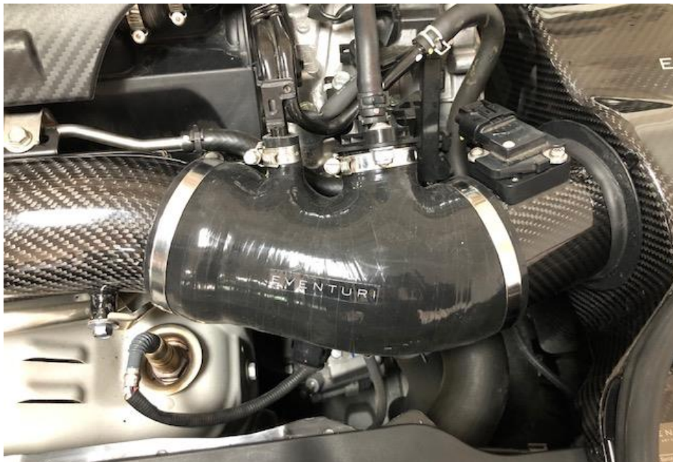
35. Install the new silicon hose.
