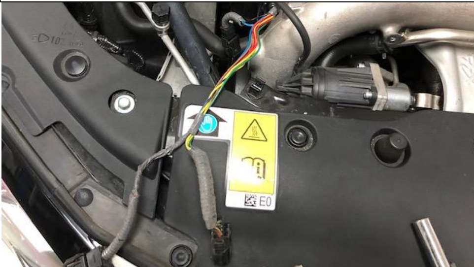
11. Remove the cover completely to leave the exposed wires.
