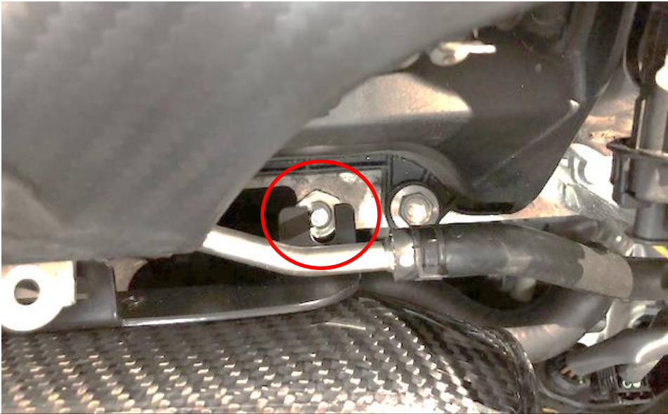
29. Rotate the tube to locate the bracket onto the anti-vibration mount. The bracket should sit flat on top of the mount.
