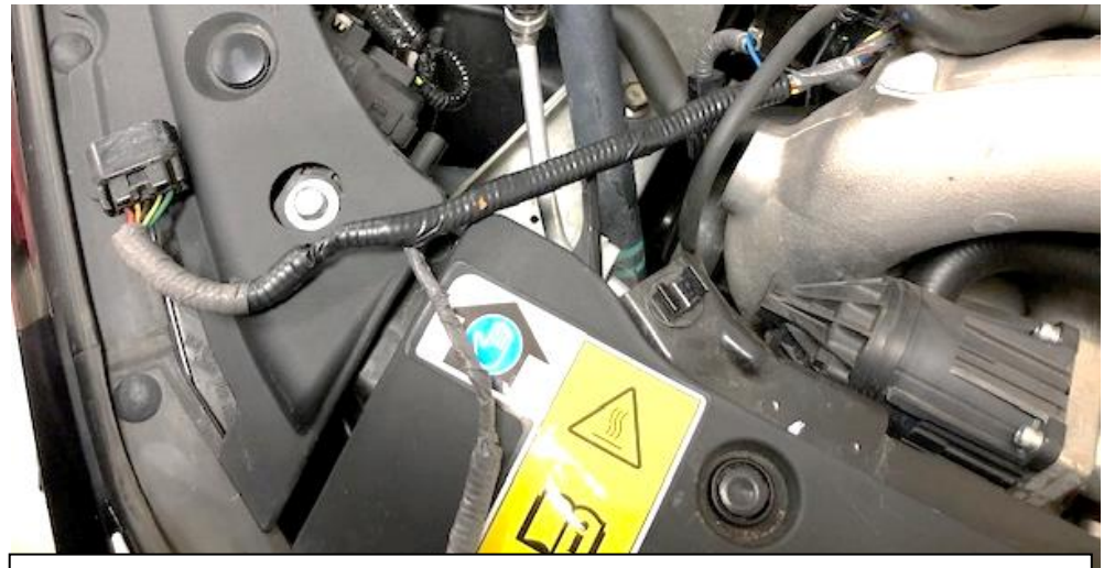
12. Use the supplied protective cable conduit and push the wires inside it. Cut to required length. The piece you cut can be used for the small length of wire which branches off. Tape around the conduit with electrical tape so that the wires are fully enclosed.
