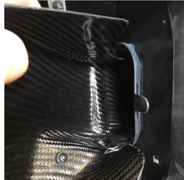
36. Push the scoop down so that it locates inside the stock duct as shown. Your scoop installation is now complete. Push the grill back into the bumper.
