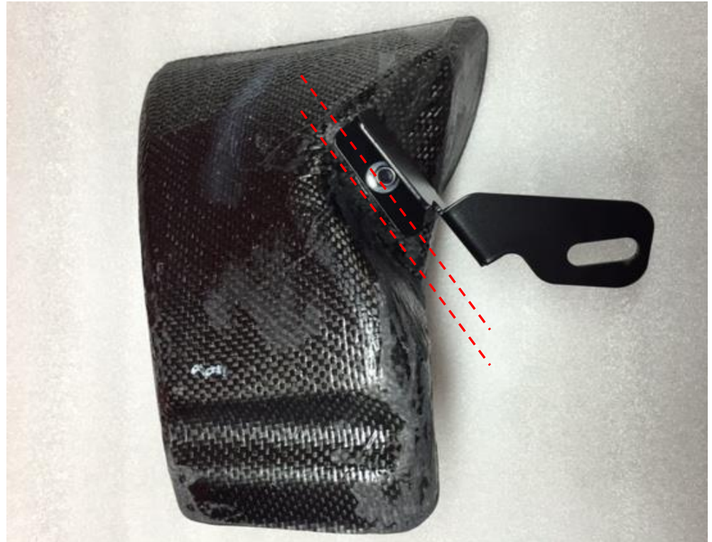
30. Take the metal bracket and mount to the back of the scoop through the screw as shown. Secure with a washer and lock nut. Orientation should be as shown with the edge of the bracket parallel to the edge of the slope on the carbon scoop.
