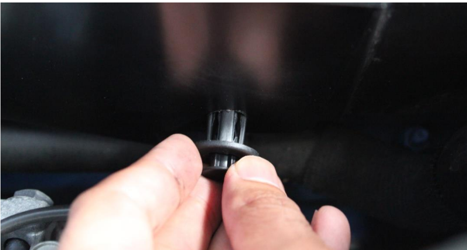
11. Push the rivet through one of the holes on the duct previously aligned in step 9. The rivet must be oriented so that one of its legs is facing upwards as shown.
