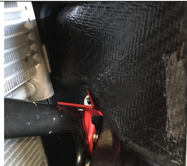
38. Now secure the bracket to the brace by using the supplied M6x20 bolt and lock nut (see step 24). Bracket shown in red for illustration. Push the grill back into the bumper.
