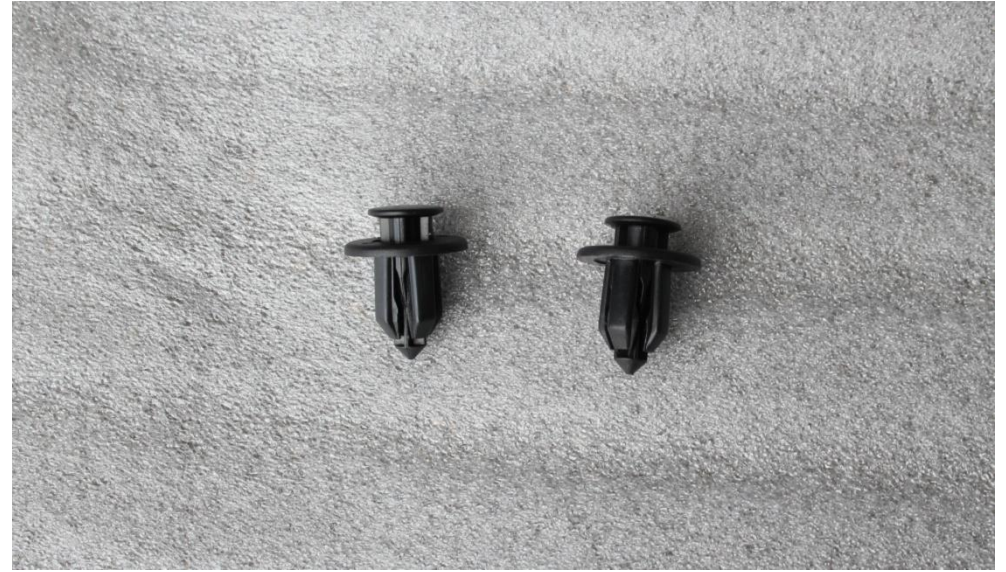
10. Take the 2 plastic push rivets supplied – these will secure the metal duct in place.
