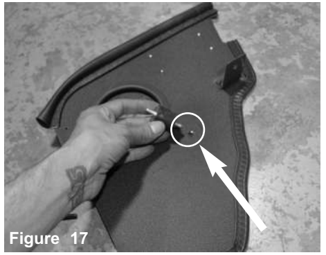
Figure 17 With provided M6 vibramount, install to the threaded insert on the back of the passenger side heat shield. Secure and tighten.
