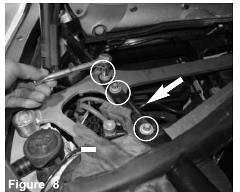
Figure 5 Loosen the engine tray and pull back weather trim seal.
