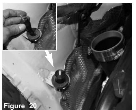
Figure 20 With provided M6 stand off stud, locate the factory OEM grommet location on passenger side, install and secure the stand off stud to the grommet. Make sure the stand off stud is seated.
