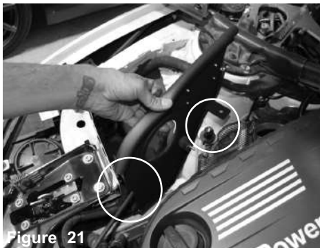
Figure 21 Install the passenger side heat shield and position the bracket to the stand off stud and front bracket to the screw from step 19.
