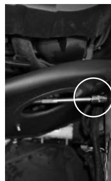
Figure 25 Position the passenger heat shield to best fit. Tighten both nuts using 10mm socket and ratchet and 10mm wrench.
