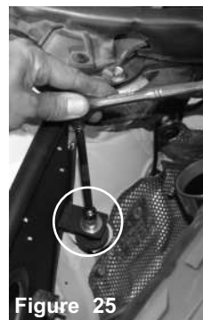
Figure 25 Position the passenger heat shield to best fit. Tighten both nuts using 10mm socket and ratchet and 10mm wrench.
