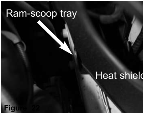
Figure 22 NOTE: Make sure the heatshield sits inside of the Ram-scoop tray. It will not install correctly if the heat shield sits outside of Ram-scoop tray.
