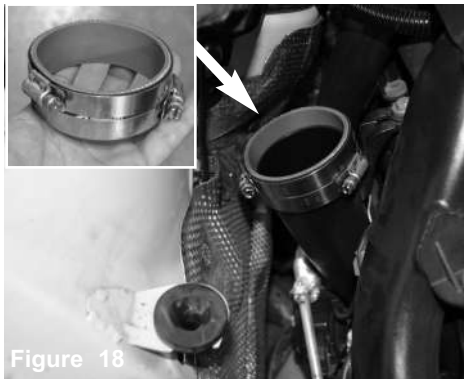
Figure 18 Place clamps to 3" hose like above image for easy access when securing the clamps. Now install the hose assembly to the turbo housing. Tighten the clamp on the housing only using 8mm nut driver.
