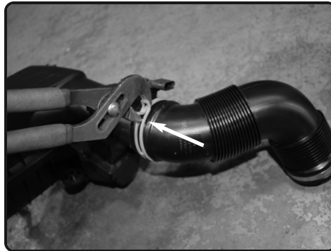
5. With pliers carefully pull back the clamp.
