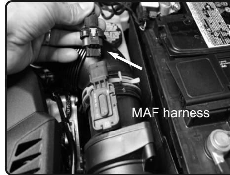
7. Disconnect the MAF sensor harness from the intake system.
