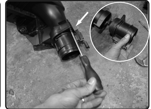
7. With T25 torx bit, loosen the 1 bolt holding in the MAF sensor. Rotate and remove the MAF sensor from the air box. Save for later install.
