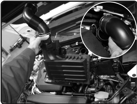
4. Pull back the intake tube from the turbo, now lift up and remove the entire intake system out of the vehicle.
