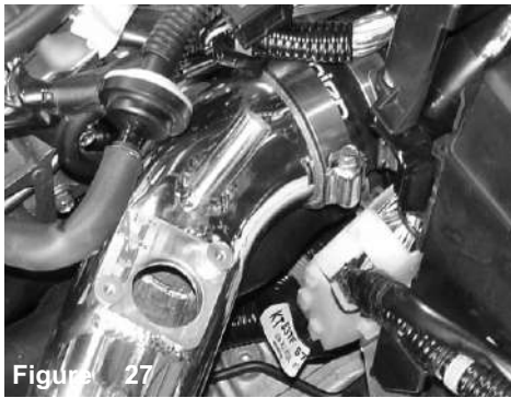
Figure 27 Once you have inserted the lower end into the bumper area, continue to press the upper intake into the step hose, semi-tighten the second power-band for now.
