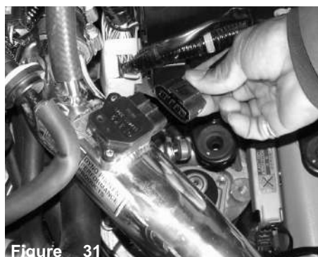
Figure 31 Press the electrical harness clip to the air mass sensor until it snaps in place.
