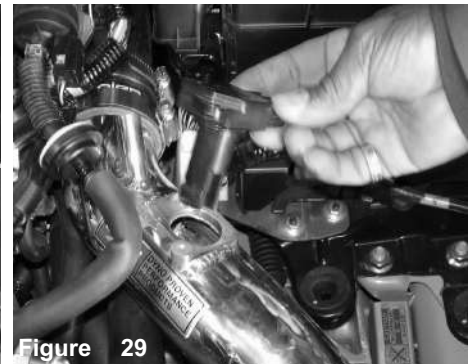
Figure 29 Prior to inserting the air mass sensor into the sensor adapter, moisten the O-ring with a light oil to prevent the O-ring from getting pinched.
