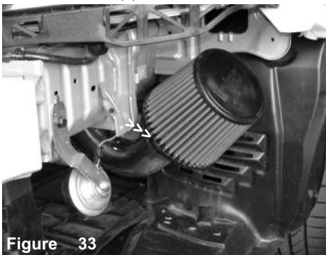
Figure 33 The tuned filter is now pressed over the end of the intake. Once the intake is butted up against the filter stop, continue to tighten the filter neck clamp.
